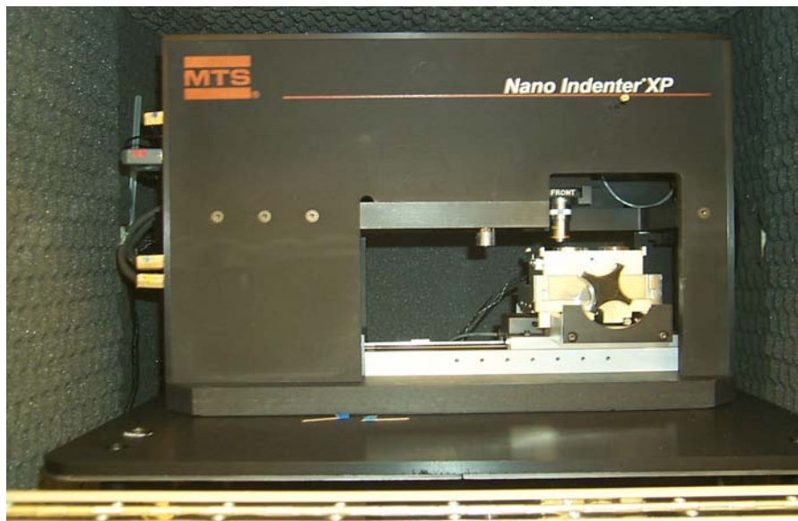
Figure 3.3 Nanoindenter used for the mechanical characterization of thin films
